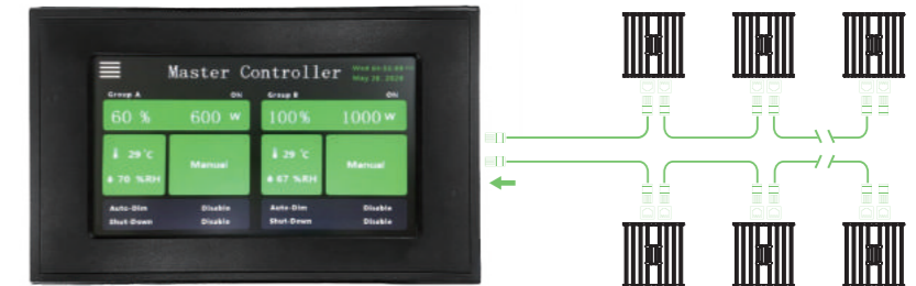
Master controller (support 1 channel 485 control signal)
